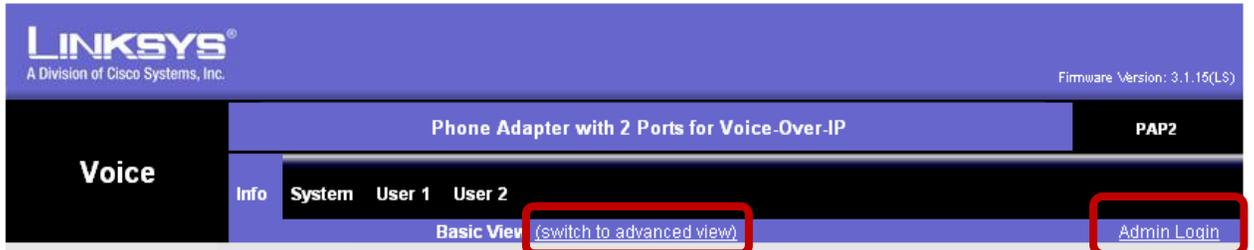
Figure 1: Admin Login and Switch to Advanced View
