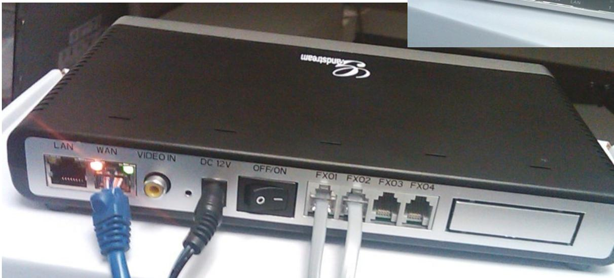
2. Make wiring connections to the LAN per the photo above – Connect the Grandstream **WAN** port to an available LAN port of the network switch/router being used on site.
